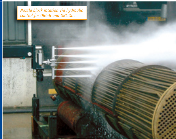
Horizontal and vertical rotating nozzle bar via two hydraulic motors.
