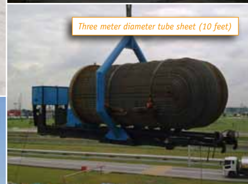
100T bundle puller with 100T winch capacity
