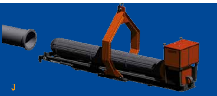
When slings are loose, disconnect and remove extractor
