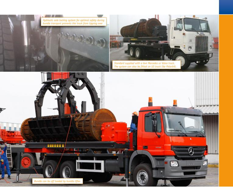
Being road legal and self contained, the Truck Mounted Extractor is a versatile and efficient tool. Exchangers residing beneath pipe rack or other structure are easily accessed with this extractor.
